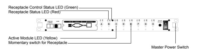
**Receptacle Status LED (Red)**: When the LED is illuminated the receptacle is on and providing AC Power. When the LED is off the receptacle is not providing AC Power.
